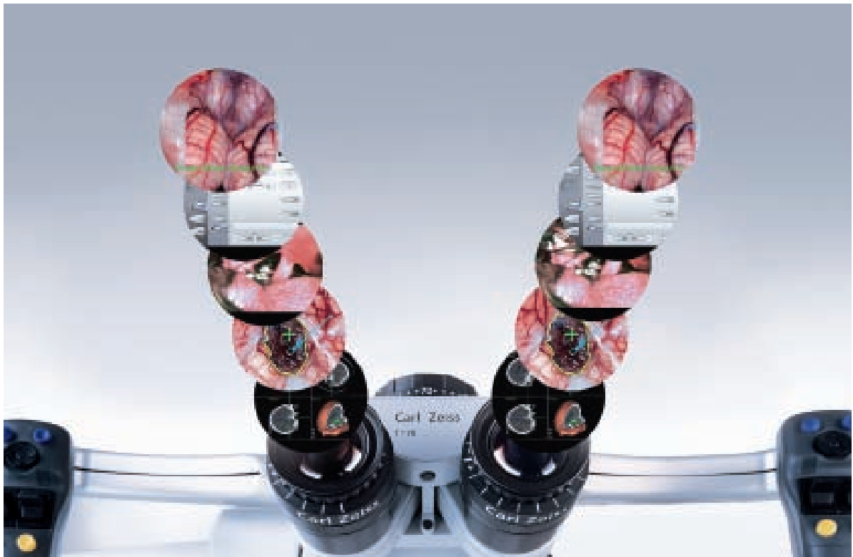
Fig. 3: MultiVision enables the surgeon to superimpose color contours and data into both eyepieces of the surgical microscope. Moreover, video data, pre-operative data, endoscope images as well as the entire touchscreen interface can be injected into the MultiVision display.
